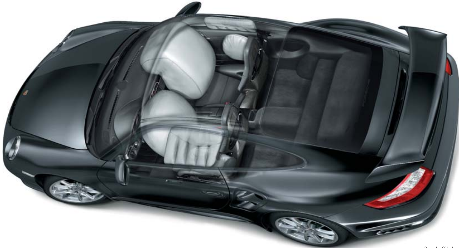
Porsche Side Impact Protection System (POSIP)
