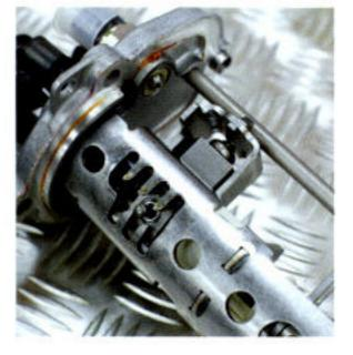
ALL M12 GTO-3RS HAVE THE LATEST GETRAG-FORD SIX-SPEED GEARBOX, WHICH IS CONTROLLED BY A SLICK AND SHORT-THROW GEARSHIFT, CLOSER INTERMEDIATE GEAR RATIOS OFFER IMPROVED ACCELERATION, WHILE A HIGHER TOP GEAR ALLOWS LOWER ENGINE REVS AT CRUISING SPEEDS, MEANING BETTER FUEL CONSUMPTION AND LESS ENGINE NOISE.
