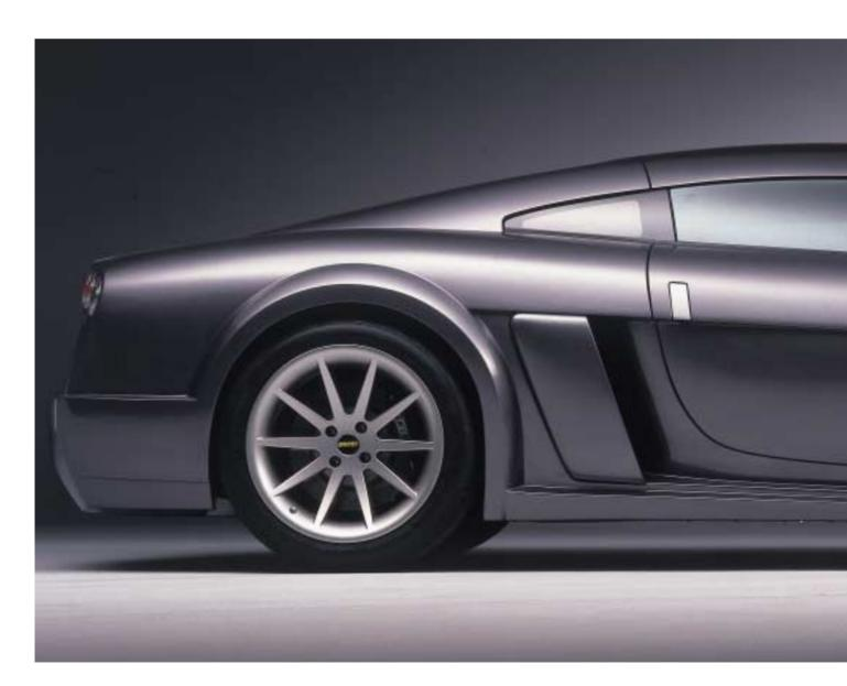
Twin intercoolers now feature in the M14, and are mounted behind each rear wheel arch. This location has two clear advantages: it creates vital space at the back of the car for a luggage compartment; and cooler air can now be ducted over each internal wheel arch cover, rather than above the engine, improving the efficiency of the intercoolers.
