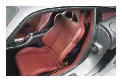
The stunning and sumptuous seats, which will be standard in all M14s are manufactured specifically for Noble. They feature a carbon fibre frame, for strength and lightness, and are trimmed in the same top-grade leather seen elsewhere in the cabin. Both seats incorporate fore and aft adjustment, as well as reclining backrests and tilt adjustment.
