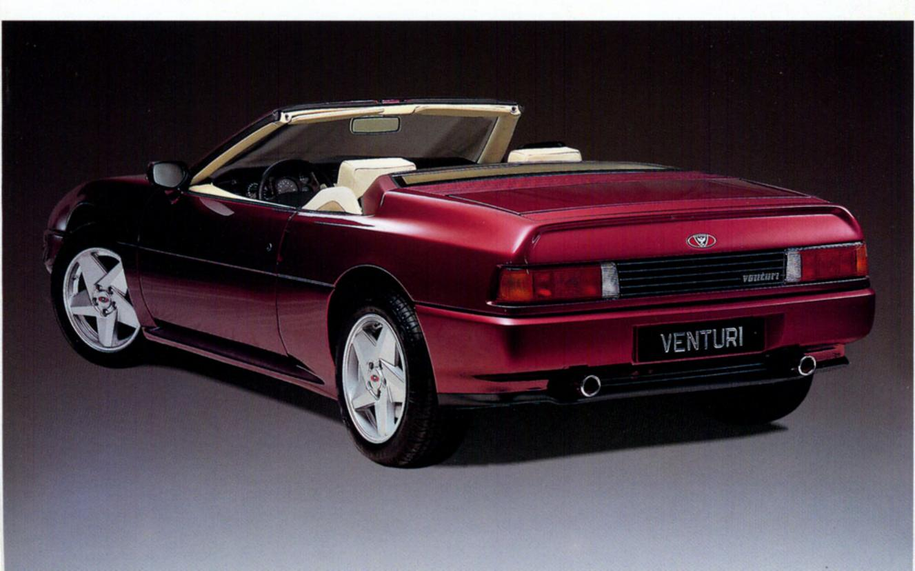
The Atlantique is a "no holds-barred" Venturi with weight trimmed by 100 kg to boost performance. Everything has been modified: from the smallest bolt to the shock absorbers, sheet metal has been replaced by aluminium, the anti-roll bar
