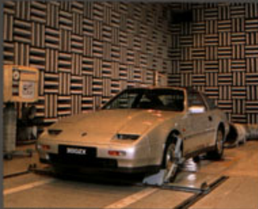
Anechoic room test
