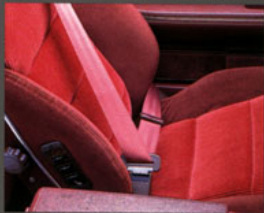
3-point hybrid ELR front seat belt
