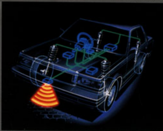
Nissan's ultra-sophisticated electronically controlled suspension automatically alters its damping rate in accordance to road and running conditions.
