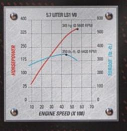
LS1 specifications include an allaluminum block designed for stiffness,
