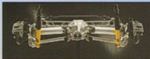
FULLY INDEPENDENT REAR SUSPENSION A unique 5-link independent rear suspension with a transverse monoleaf spring helps put power to the pavement.
