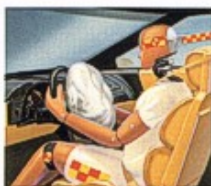
A driver's-side Supplemental Inflatable Restraint (air bag) is located in the hub of the steering wheel. The S.I.R. is designed to provide added protection to the
