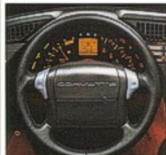
The new-for-1990 Supplemental Inflation Restraint system (air bag) is located in the hub of the steering wheel. The S.I.R. is designed to provide added protection to the driver in the event that your Corvette is involved in a moderate to severe frontal impact. For maximum protection in frontal and all other collisions, both driver and passenger should be properly restrained with safety belts.
