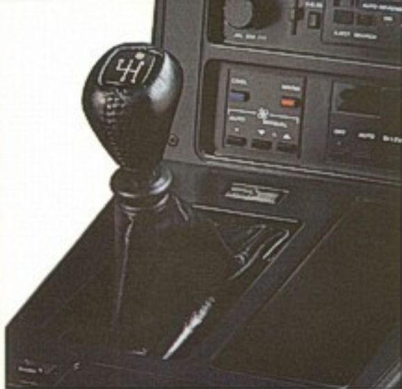
Corvette's 4-speed manual overdrive is a no-cost option. This transmission offers the unique flexibility of seven ratios, enhancing both economy and performance.
