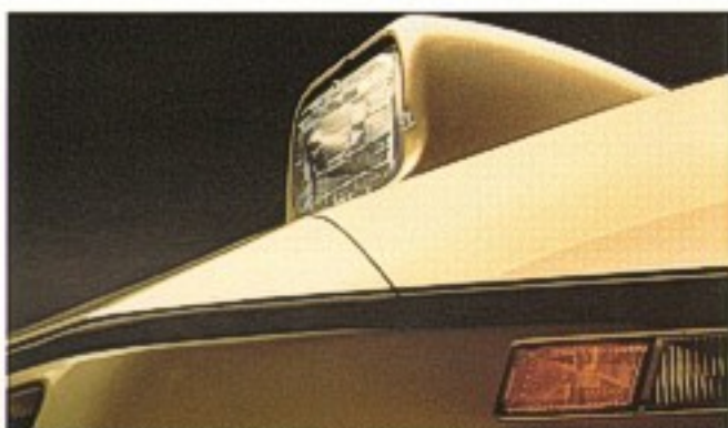
RETRACTABLE HEADLAMPS FLIP FORWARD 162.5 DEGREES FROM BENEATH THE HOOD.
