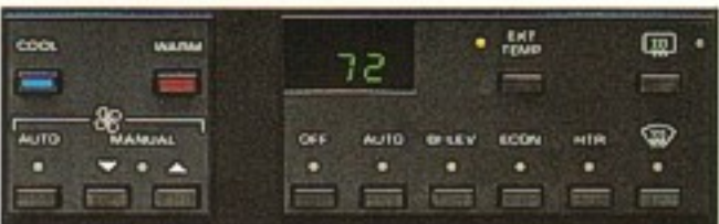
ELECTRONIC AIR CONDITIONING FEATURES FINGERTIP PUSH-BUTTON CONTROL.
