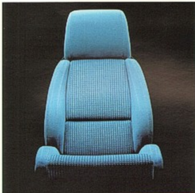
AIRCRAFT-COCKPIT-STYLE HIGH-BACK CONTOUR SEATS WITH MANUAL BACK ADJUSTMENTS AND BOLSTERS TO PROVIDE SIDE SUPPORT ARE UPHOLSTERED IN ATTRACTIVE CLOTH.
