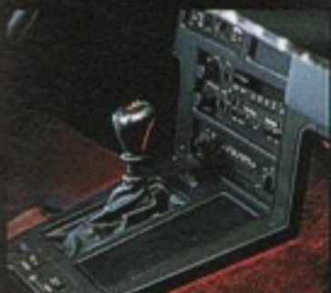
Four-speed manual transmission features electronic overdrive in top three gears.
