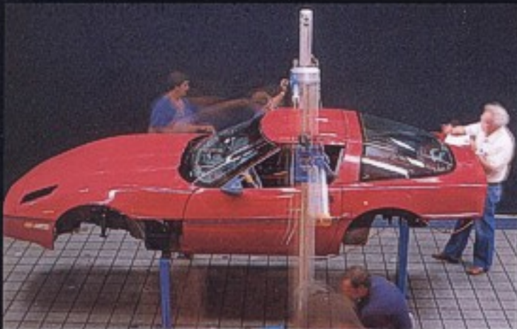
Point-check inspection to make sure body panel assembly meets design intent.
