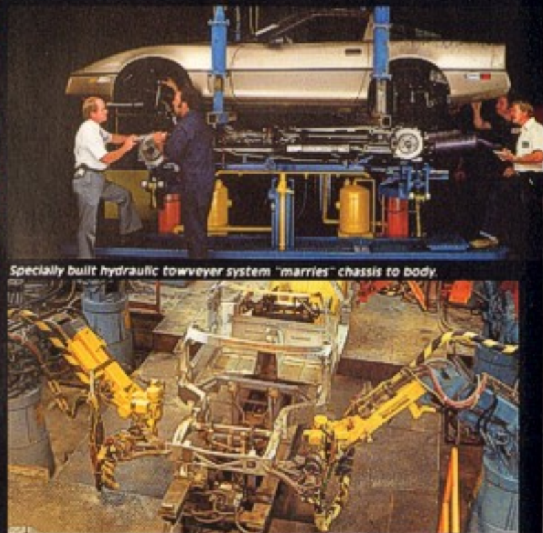
Uniframe components get additional precision robot welds.
