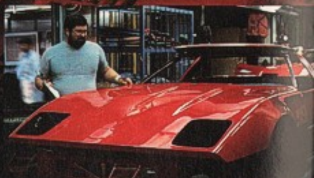
Meticulous wet and hand sanding are demanded by Corvette's tough paint inspection standards.
