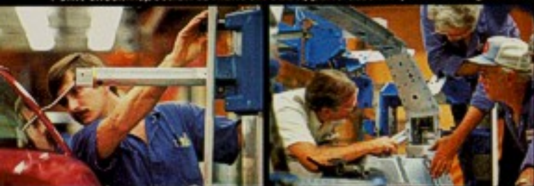
12 Technicians use computerized instruments to measure body panels to close tolerance on three planes.
