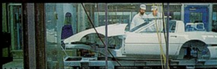
Between-coat inspection of Corvette paint.
