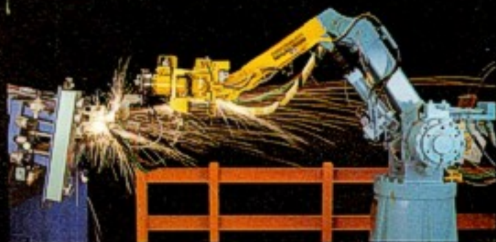
Uniframe components get additional precision robot welds.
