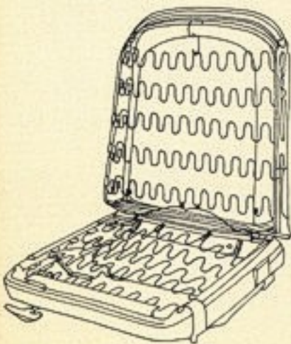
S-wire spring construction
