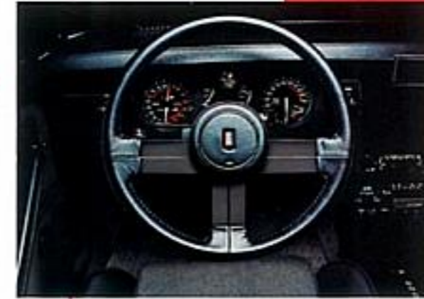
Above: Z28's new optional L/S Contour driver's seat. Left: Z28's instrumentation includes tachometer, trip odometer, voltmeter, temperature and oil pressure gages.
