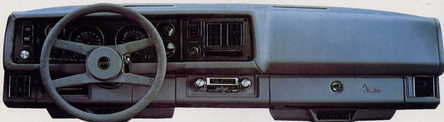
Camaro Z28 instrument panel shown with available electric rear window defogger, AM/FM stereo radio with 8-track stereo tape and air conditioning.
