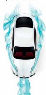
After an extensive programme of advanced computer simulations, the Supersports' engineering team calculated that an increase in turbocharger boost would require a 10 percent increase in airflow to the twin intercoolers and cooling system, thus allowing the engine to generate its extra power and torque.
