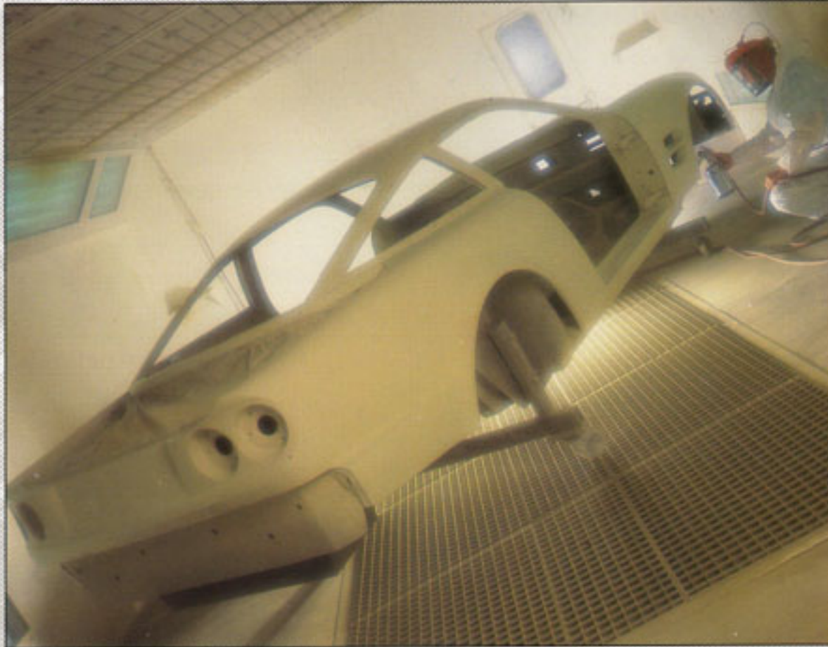
A Vantage passes through the paint system at Newport Pagnell
